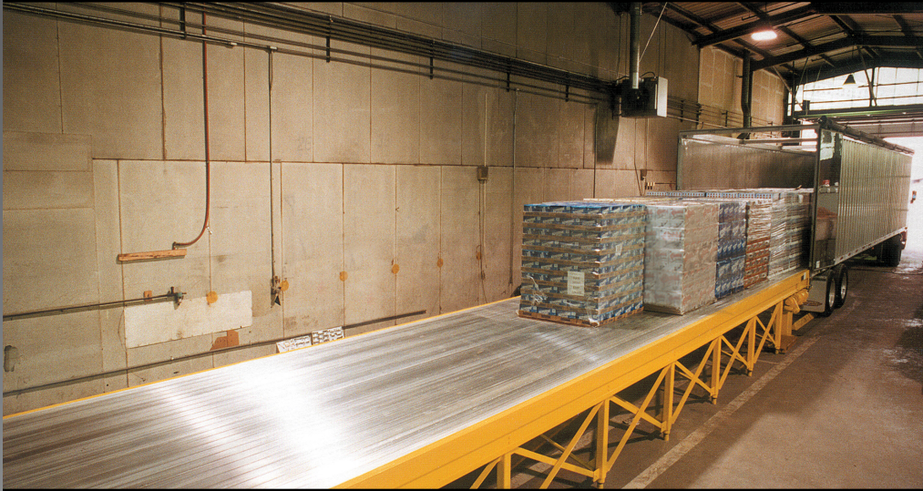
Dock and trailer slats move together conveying the load.
